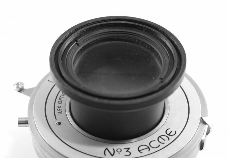
5. Thread your Ilex shutter into your Mercury mounting parts (either a shutter plate or an XL barrel, depending on the lens). Remove the Ilex shutter's retaining ring or flange first, as it will get in the way, and isn't used when mounting an Ilex No. 3 on a Mercury.
