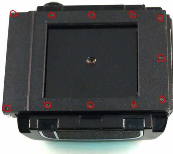
2. If it is a Pro-S style back, you will find a silver interlock also sandwiched between the two pieces. Remove the central screw (with a thin slotted screwdriver), then carefully remove the metal arm and spring.
