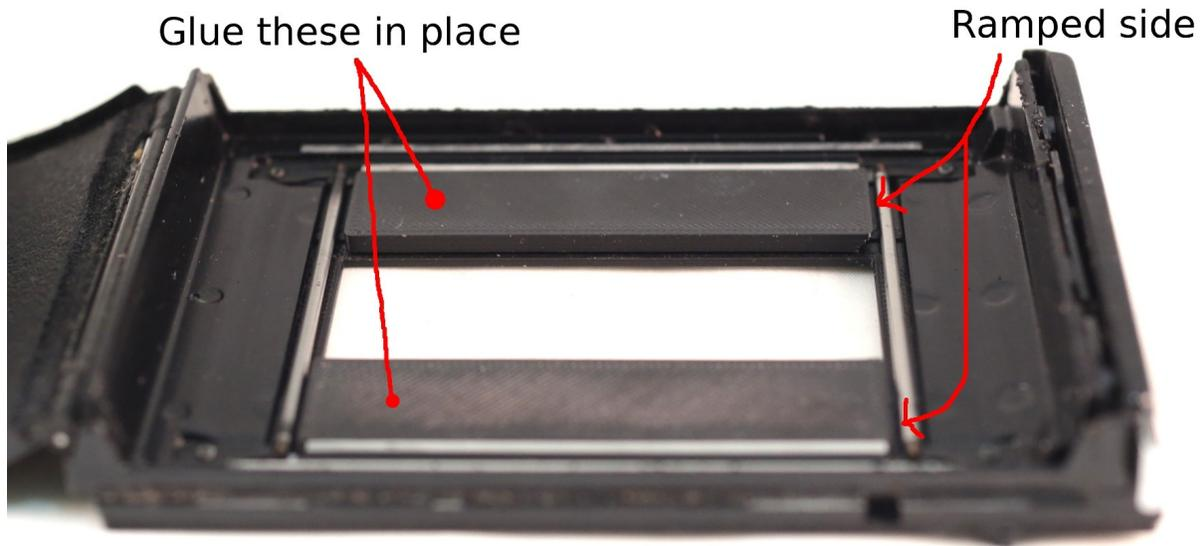
While the glue cures overnight, you should place some **heavy, flat objects on top of the film guides** to ensure that they remain very firmly pressed against the Graflok plate.
