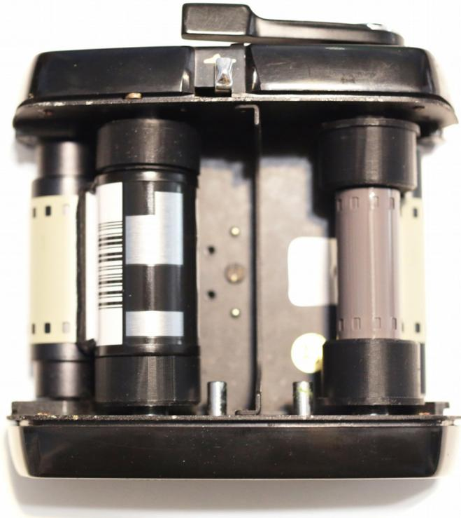
7. Replace the takeup spool with the Mercury version. This is the same size as an ordinary 120 spool, but has a thick head and base, and space for film takeup on only a smaller part of the spool (in the middle).
