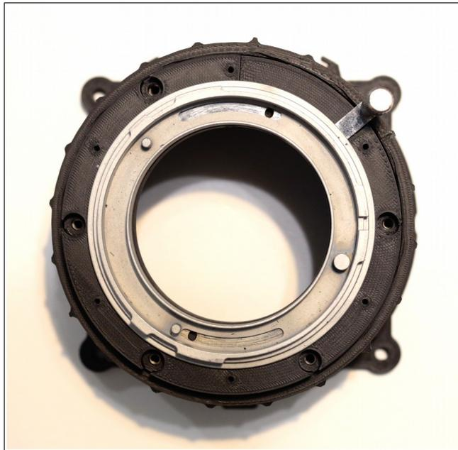
6. Screw in the six silver screws that came with your Mercury adapter kit. This will hold the top ring down and anchor the entire assembly.
