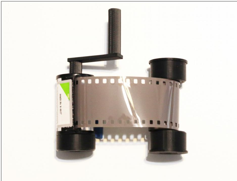
2. Remove the top adapter from the cartridge and replace it with the rewind crank.
