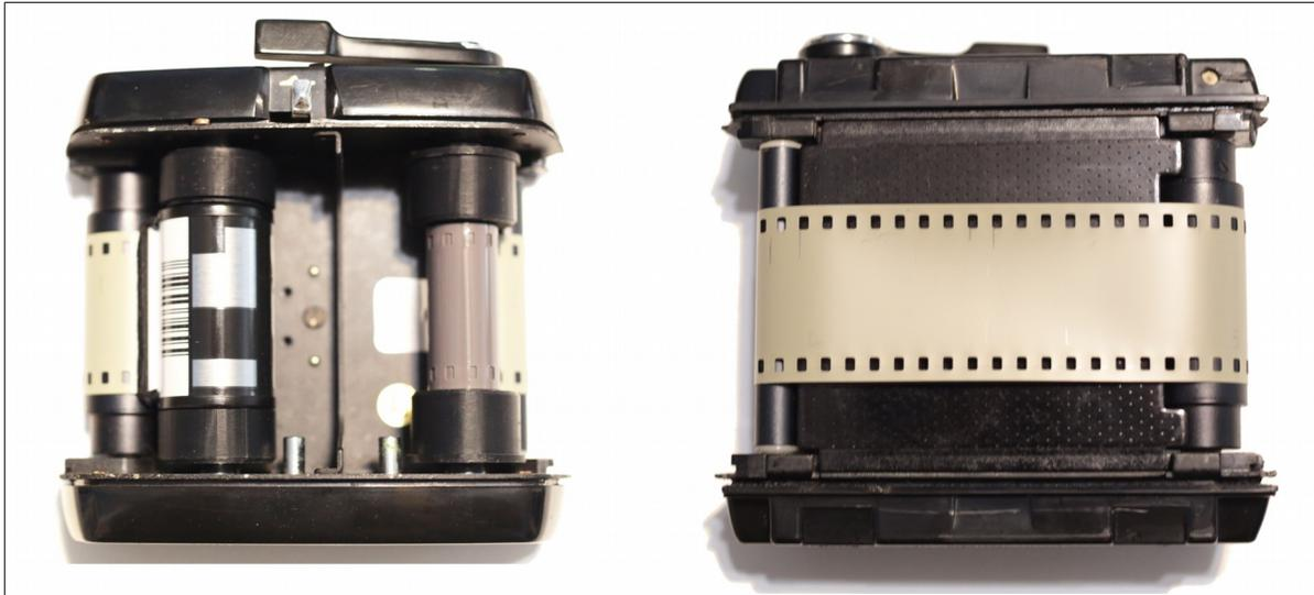
6. If you have loaded the film correctly, the dull, emulsion side of the film should be visible across the pressure plate and the shiny side down (not visible). Double check this!
